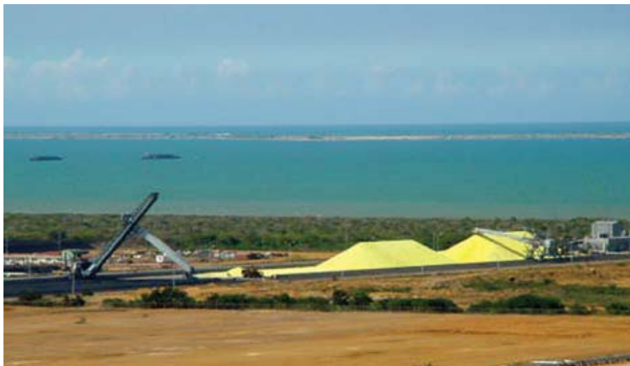
Rick Rys took this picture while working at a refinery in Venezuela. The large yellow piles are sulfur that was removed from crude oil.
